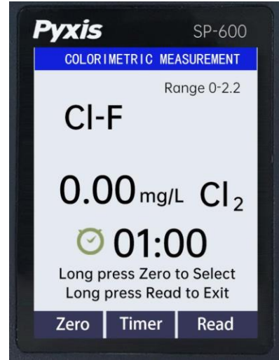
Figure 2. Zero on Figure sample before reagent step
